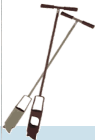
Soil bucket augers used to determine the depth of the seasonal high water table.
