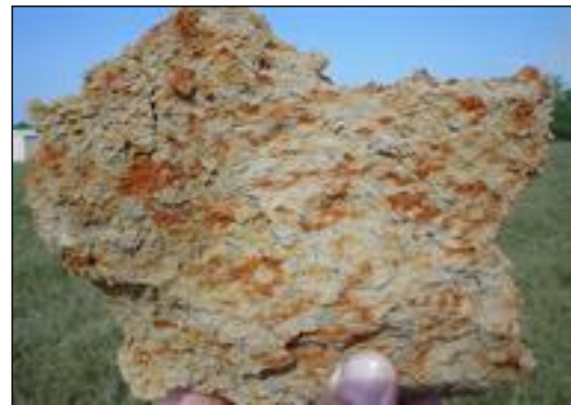
Red (concentrations) and gray (depletions) soil colors indicating the location of the seasonal high water table.
